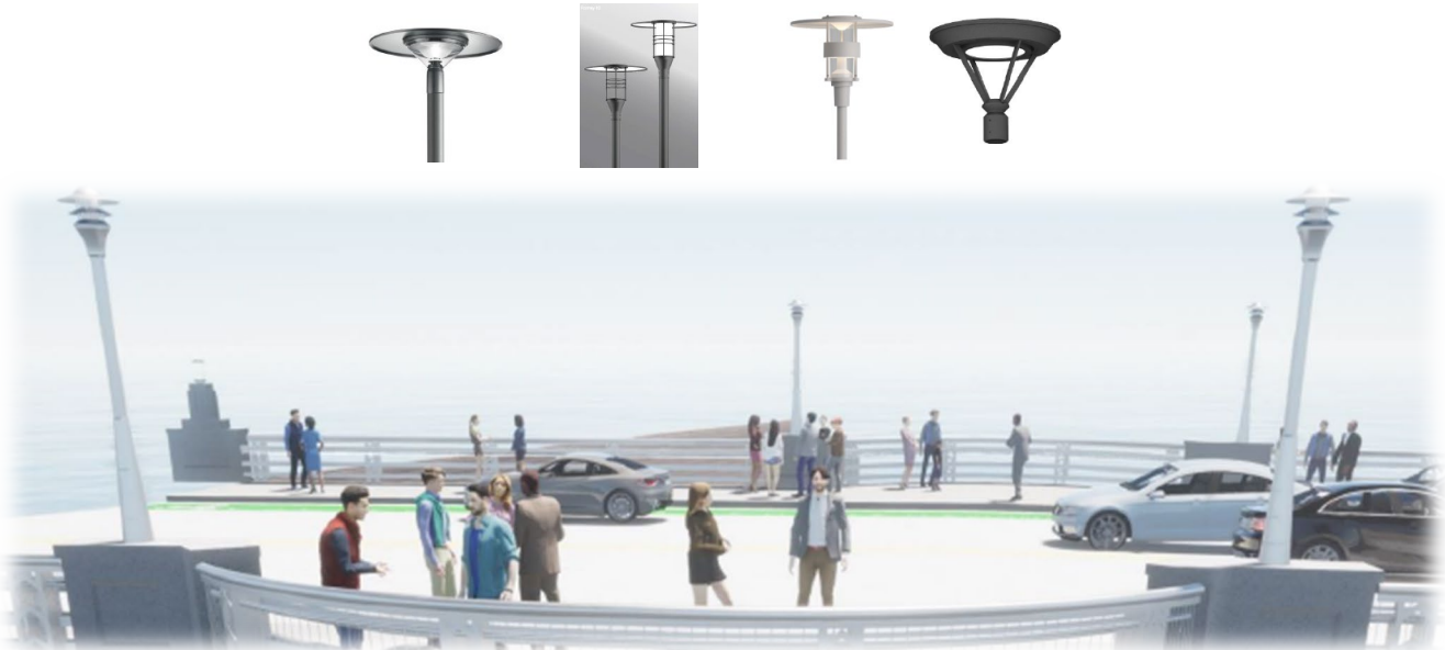
Figure 7. Pole with Post-Top Luminaire Lighting
