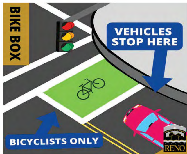
Figure 2-8 - How to use an intersection bicycle box.
