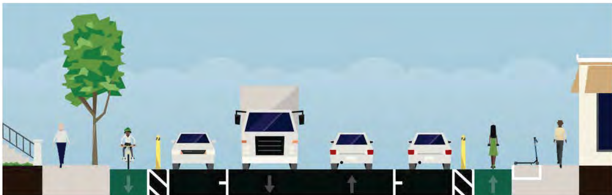
Figure 2-3 - Cross-section showing micromobility lane with parking buffer.
