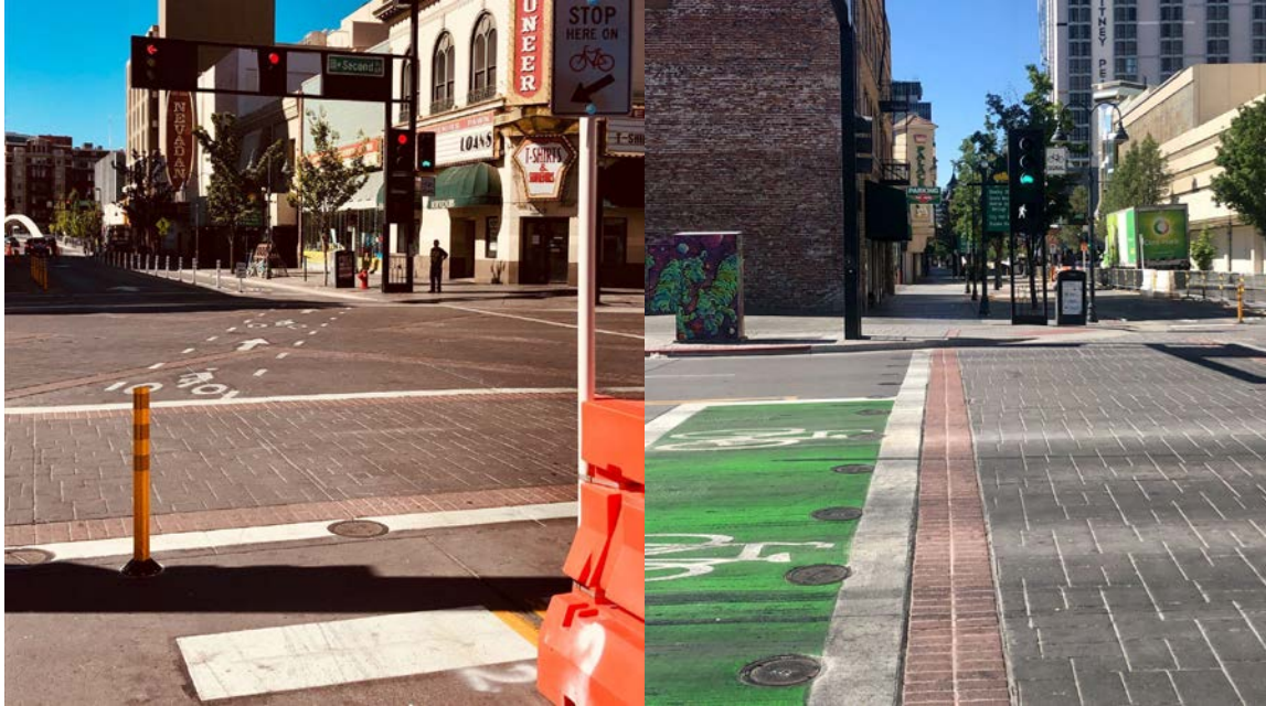
Figure 2-9 - Photos of Bike Signal at Virginia Street and Second Street and Bike Box at Fifth Street.
