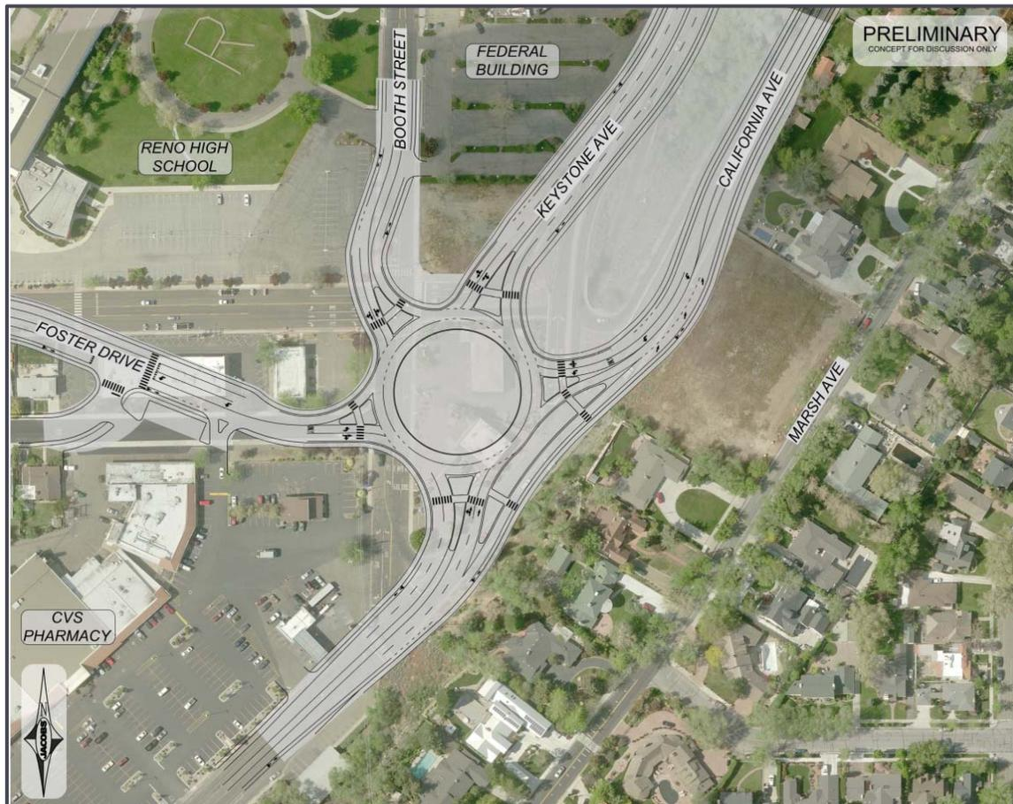
**Alternative B** replaces the existing High-T style intersection at California Avenue / Keystone Avenue with a three-legged roundabout, and it eliminates the direct connection between Keystone Avenue and Foster Drive. One of the benefits of Alternative B is it maintains and prioritizes the major regional roadway network and better separates major traffic movements from Keystone and California Avenues from using the local street network. Features of Alternative B include:
