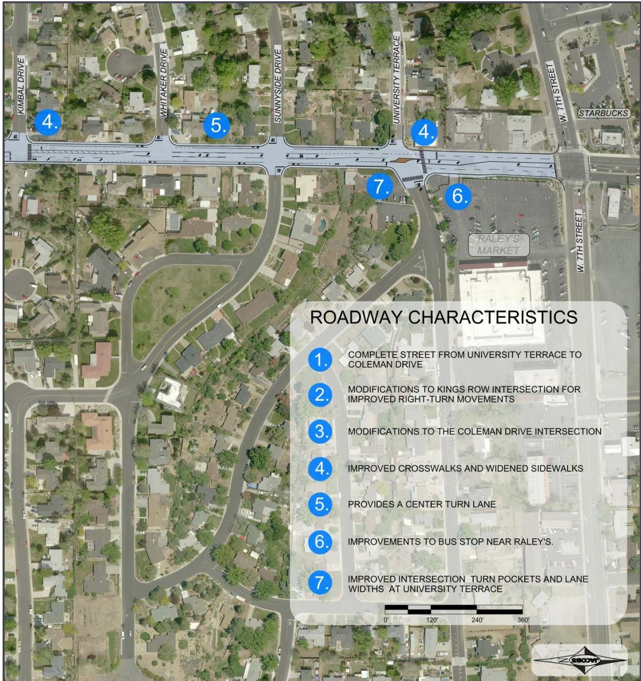
Figure 5-20: Alternative 3: Combo Alternative
