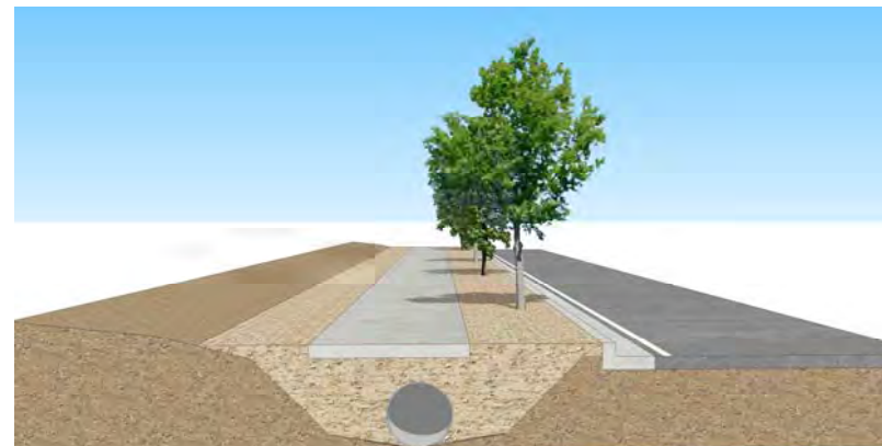
Figure 35 - Conceptual Sidewalk Installation over Existing Ditch
