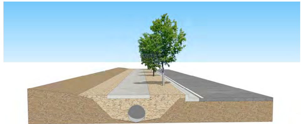
Sun Valley Boulevard - Conceptual Roadside Ditch Retrofit to accommodate sidewalk
