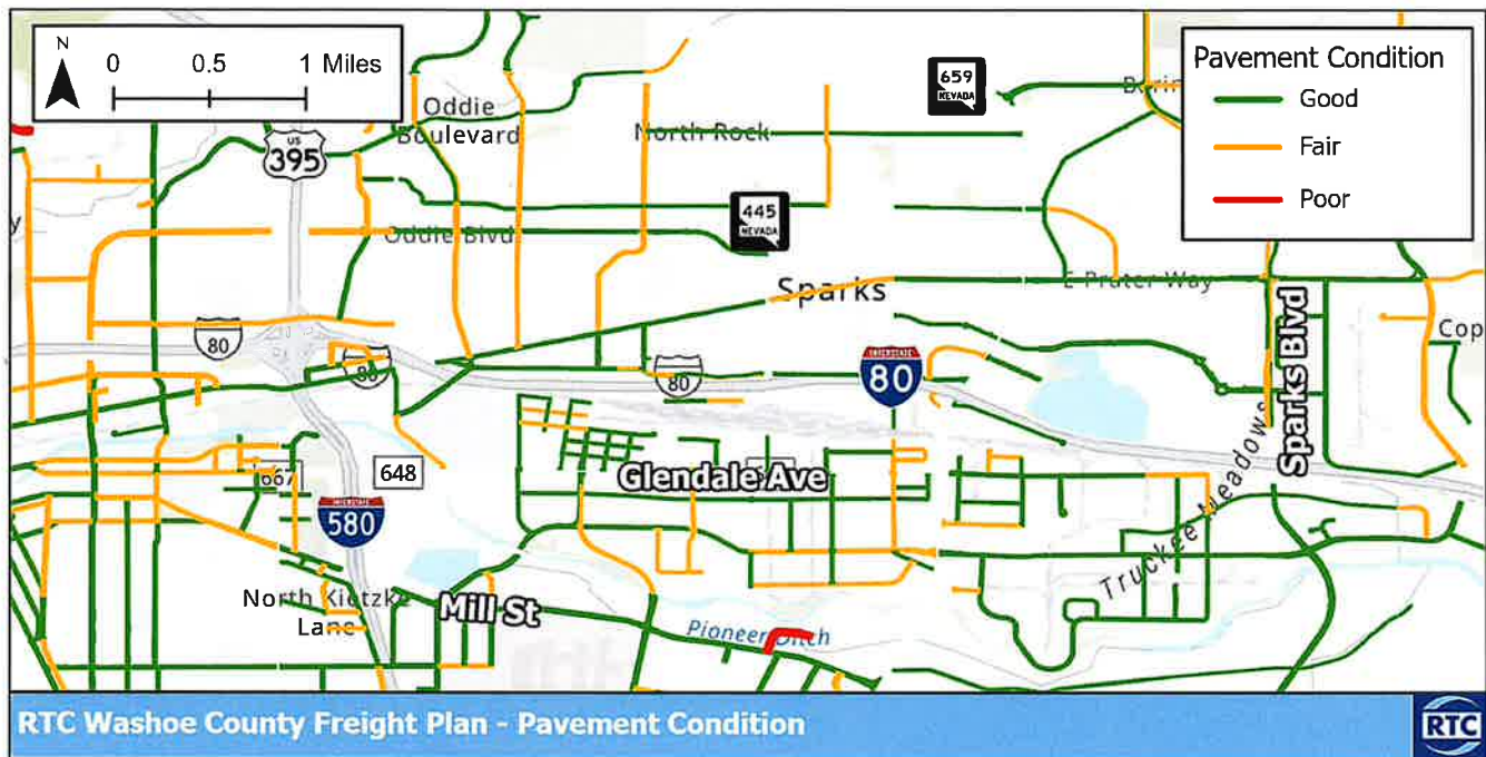
Figure 18: Pavement Condition – Sparks Industrial
