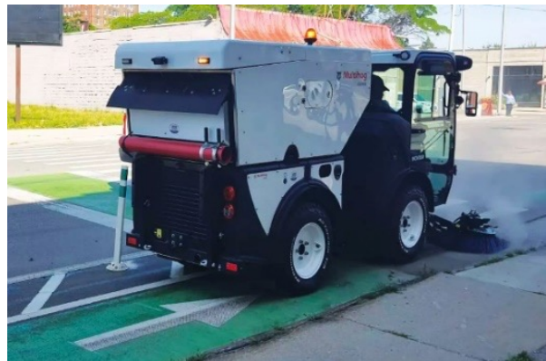
Figure 6.2 Small specialized sweeper example (Source: Multihog).
