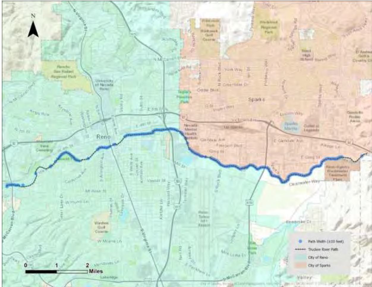
Figure 7- Path Width Meeting FHWA Recommendation (10 feet)
