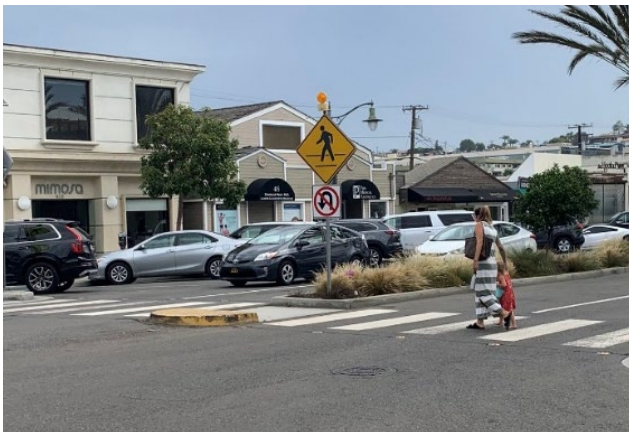
Figure 16. Pedestrian Median Refuge Island Example
